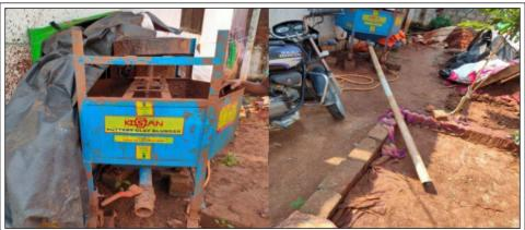
Figure 5.7: Modern Equipment Used in Making Clay Products Blunger in Hanamkonda District
