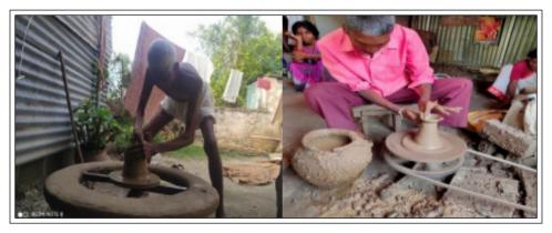
Figure 5.5: Traditional Manual Wheel in Inavole Figure 5.6: Modern Power Wheel in Ursu
